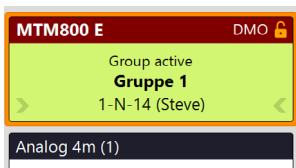
Real Names real name display of active radio users, e.g. as "Steve"
